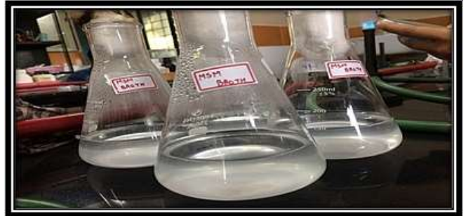
After incubation extraction was carried out by washing the MSM broth containing organism with Ethyl acetate and Methanol (4:1) for three times an organic layer was formed over the surface of MSM media.
