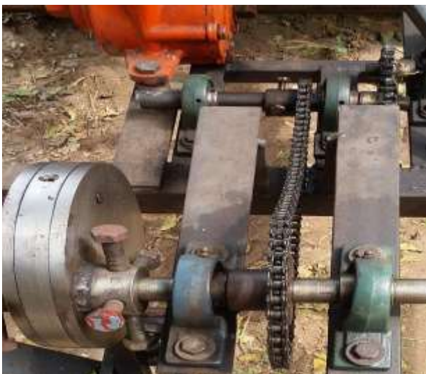
Plate-2 Final reduction transmission system (Chain and sprocket)
