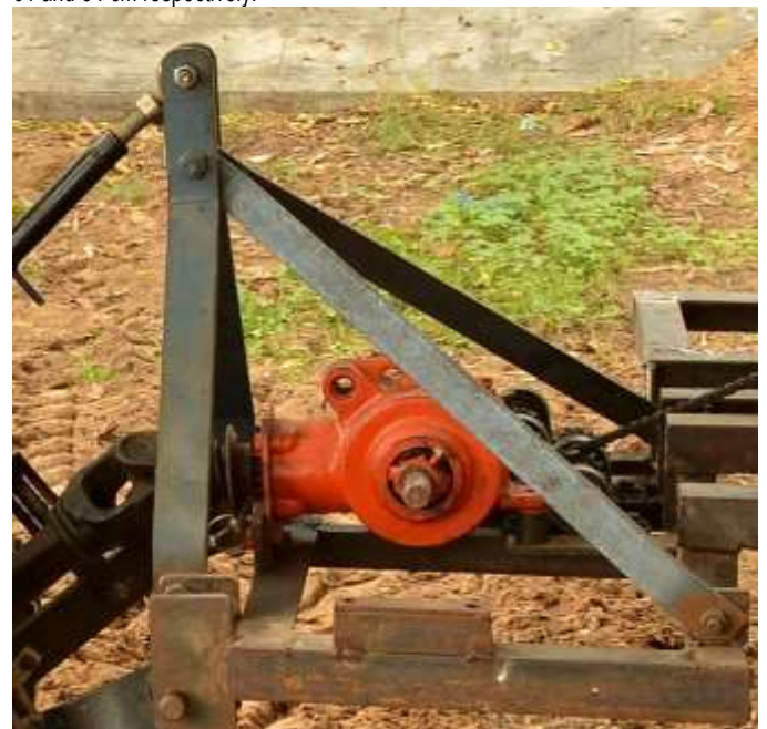
Plate-1 Three points hitch connections on punch planter
