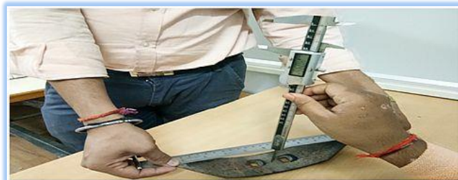
Fig-2d Measuring Concavity with Vernier calliper
