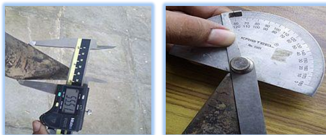
2b Measuring width with Vernier calliper, 2c Measuring Rake angle with Angalometer
