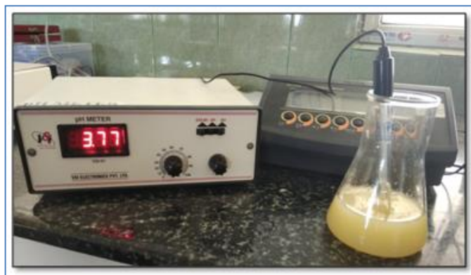
Fig-4 Measurement of pH using digital pH meter.
