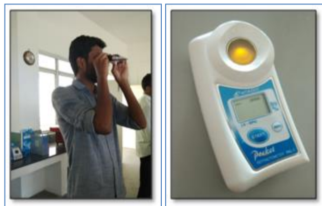
Fig-5 Measurement of TSS using refractometer.
