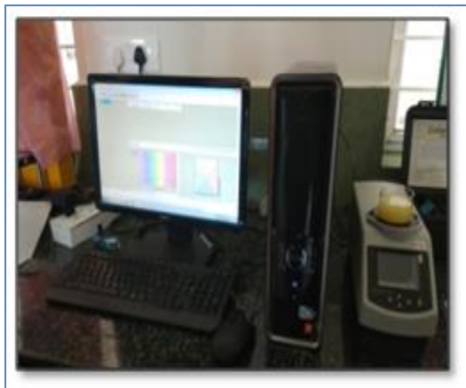
Fig-6 Measurement of color using hunter lab colorimeter.
