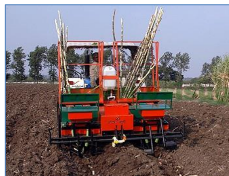
Fig-5 IISR Sugarcane cutter cum planter in operation
