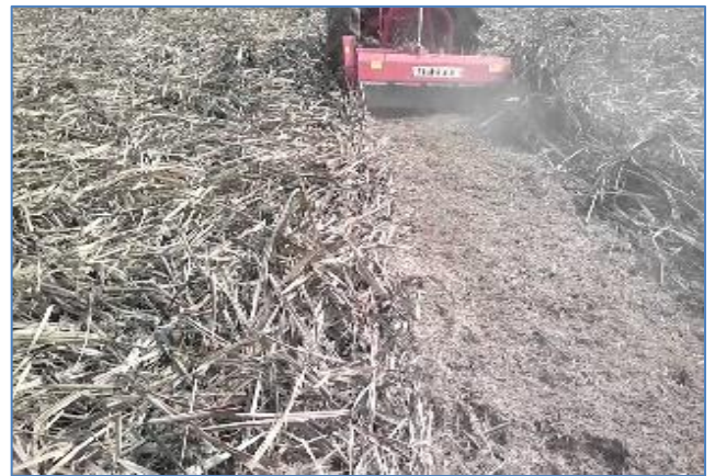
Fig-20 Sugarcane trash shredder in operation
