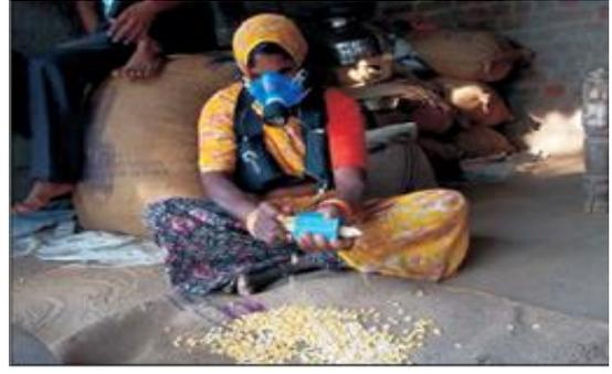
Plate 1: Measurement of heart rate and energy expenditure during maize shelling activity with the help of maize sheller
