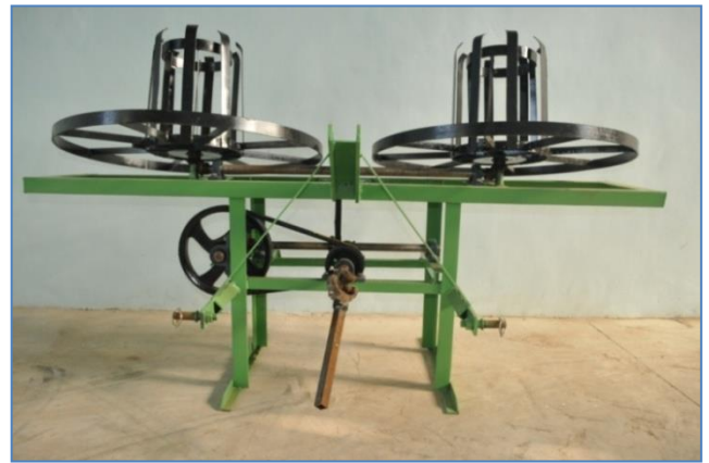
Fig-3 Prototype tractor drawn drip lateral coiler machine.
