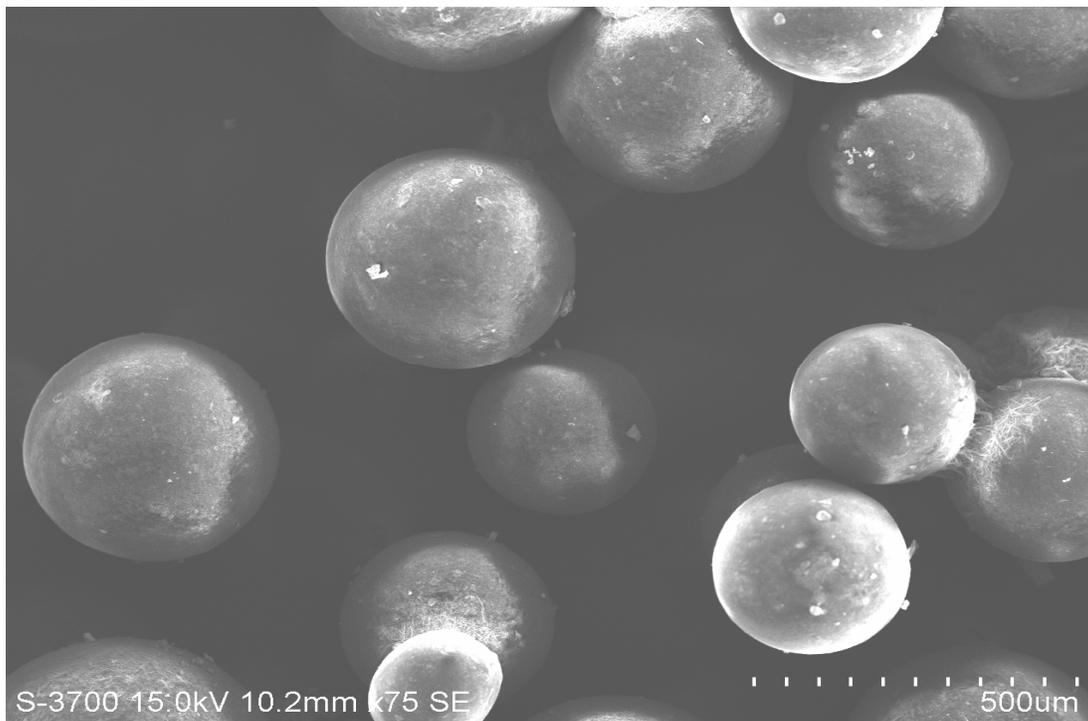
Fig. 2- SEM of ethyl cellulose magnetic microspheres loaded with Diclofenac sodium
