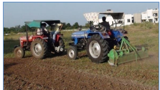
Fig-6 Draft measurement using drawbar
