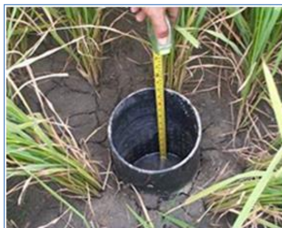
Fig 3- Water level is being measured in the fitted Pani-Pipe
