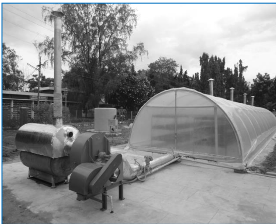
Fig-1 Solar tunnel dryer integrated with biomass hot air generation system installed at Department of Bioenergy, Tamil Nadu Agricultural University, Coimbatore
