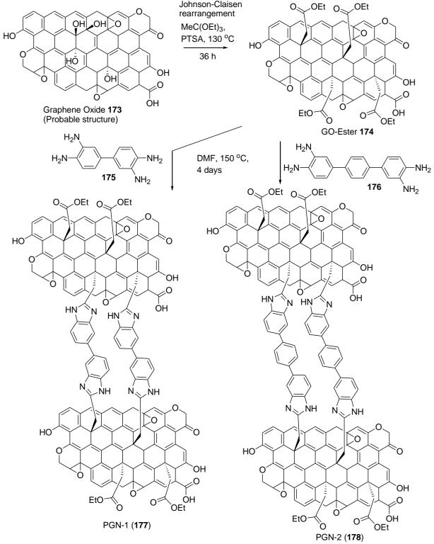
Scheme 27 Synthesis of porous graphene networks (PGNs) by Johnson-Claisen rearrangement
