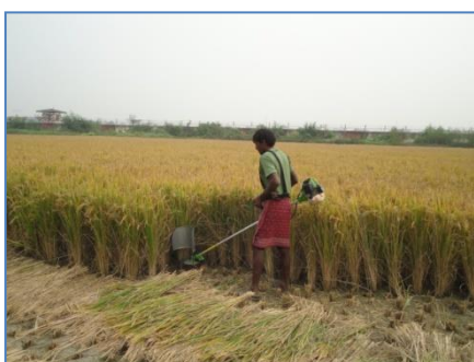
Fig-3 Testing of the crop cutter for rice harvesting at ICAR Research Complex Farm, Patna
