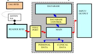
**Fig. 2-** System block diagram. Note that blue background blocks are the main constituents of the project, instead yellow background ones handle data processing. In red the main path of RFID data
