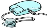
Fig. 2- Possible new mechanical design of the internet tele-stethoscope, alternatively to the classical chassis
