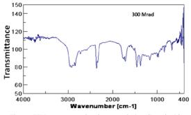
Fig. 4. FTIR spectrum for the sample irradiated with a dosage of 300 Mrad
