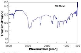
Fig. 3. FTIR spectrum for the sample irradiated with a dosage of 200 Mrad
