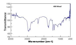
Fig. 5. FTIR spectrum for the sample irradiated with a dosage of 400 Mrad
