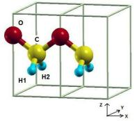
Fig. 1. Structural pattern of non fluorinated Polyformaldehyde
