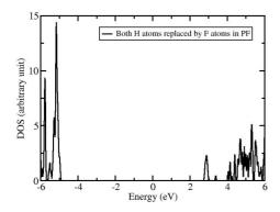
Fig. 4. EDOS in completely fluorinated Polyformaldehyde
