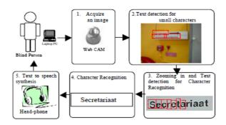
The system works as follows a) Acquire the image. b) Oriented text detection from the acquired images. c) Store the detected text. d) Character Recognition e) Text to speech recognition. This research work is intended to carry out the second step of the proposed system i.e. Oriented text detection from the acquired image.
