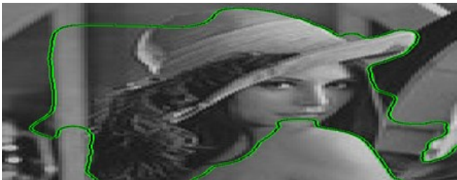
Fig. 7- Window showing effect on percentage of accuracy using Localized Segmentation with No. of iteration 500, \alpha=0.6 and \rho=32
