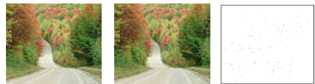
Fig 5.5- a) Original copy (b) Marked copy with 89-Bytes embedded in (c) Difference between original and marked image
