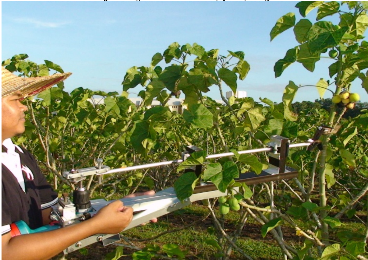
Fig. 2-The prototype shaker was attached on the tree twig for shaking.
