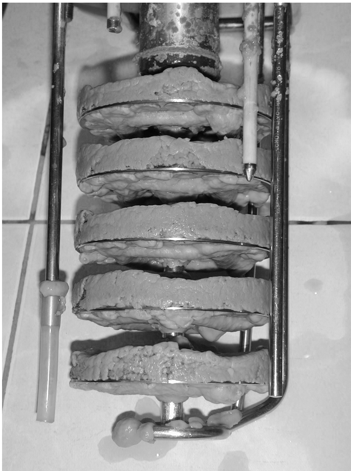
Fig. 2- Mycelium of Aspergillus niger 20 Osm immobilized on polyurethane foam disks installed on the agitation drive shaft of a Biostat B bioreactor.
