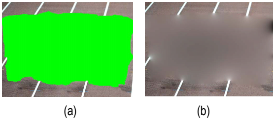
Fig. 1- (a) the masked image; (b) the image inpainting results by PDE-based
