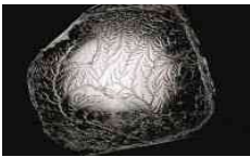
Fig. 3- A fractal is formed when pulling apart two glue-covered acrylic sheets
