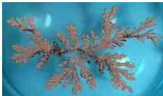
Fig. 4- A DLA cluster grown from a copper (II) sulfate solution in an electrodeposition cell
