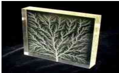
Fig. 6- High voltage breakdown within a 4" block of acrylic creates a fractal Lichtenberg figure.
