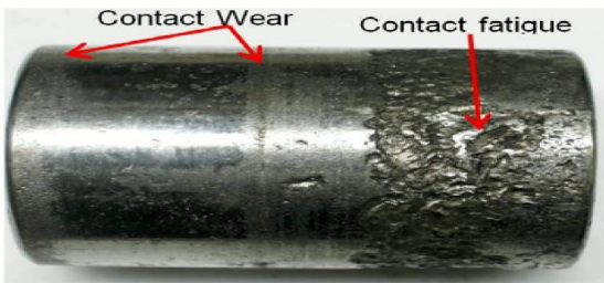
Fig. 9- Wear on roller
