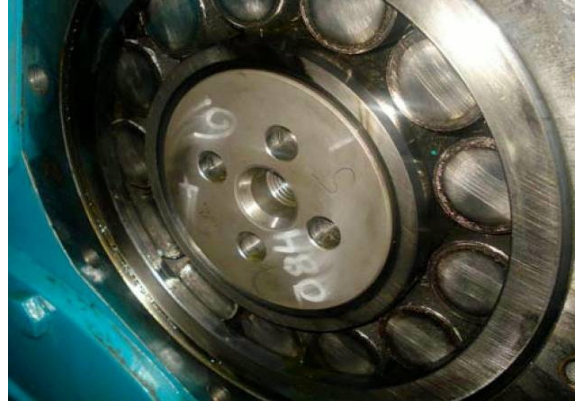
Fig. 5- Failed intermediate non-drive end bearing INA LSL 19 2330 A0993
