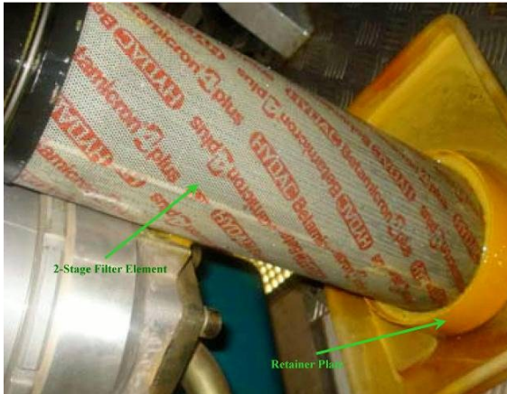
Fig. 3- Choked gear oil filter
