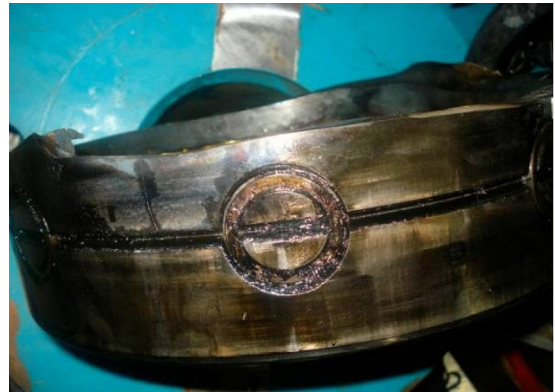
Fig. 12- Damaged outer race of bearing
