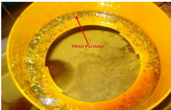
Fig. 4- Metal particles at retainer plate
