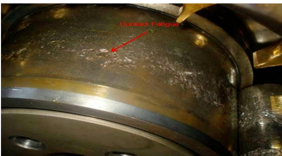
Fig. 11- Wear on inner race
