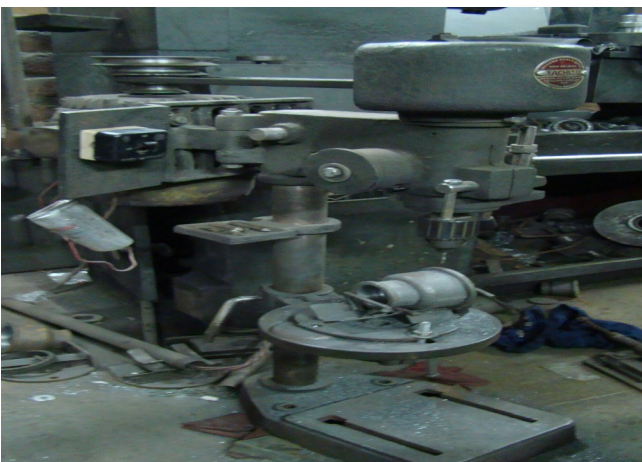
Fig. 3- A typical manually operated drilling machine which is being made automatic using virtual instrumentation system
