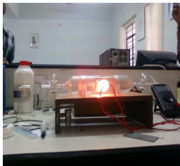
Fig. 4- Experimental setup with heating coil at 250°C
