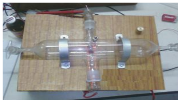
Fig. 5- Glass chamber with inlet, outlet and emergency valve at the top.
