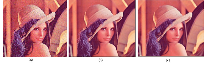
Fig. 1a- Degraded Lena image with Gaussian noise 10%, b) shows restored image by ABF and c) shows restored image by bilateral filter
