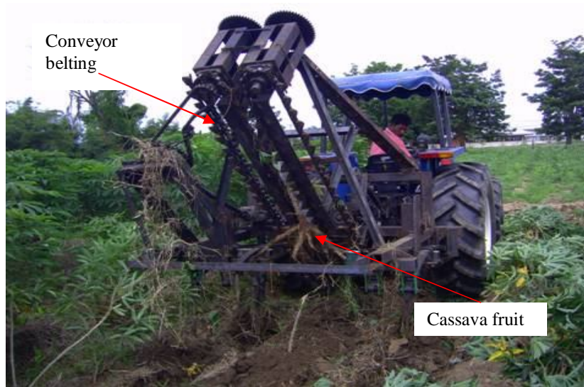
Fig. 5- Semi auto machine for cassava harvesting developed in Malaysia
