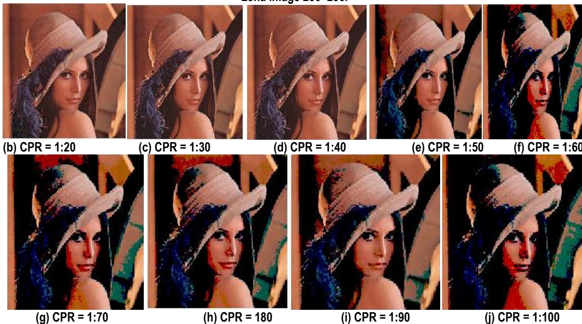
Fig. 5 (b-j) Reconstructed Lena Image for different compression ratio in Wavelet transform.
