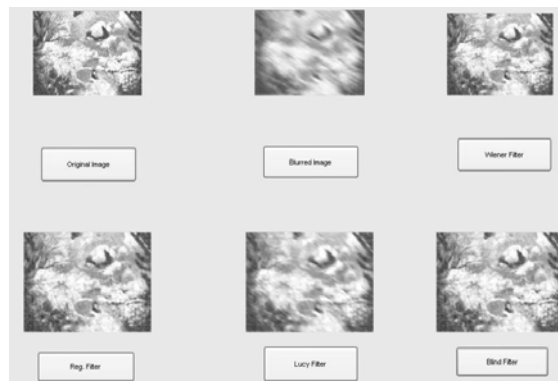
Fig. 4: Original Image with add Gaussian Noise Alfa=0.5 when PSF Known
