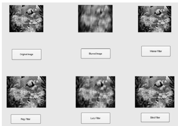
Fig. 2: Deblurring Image without add Noise When PSF Known, Image Blurred by Motion Blurred Length =10 and Theta=50
