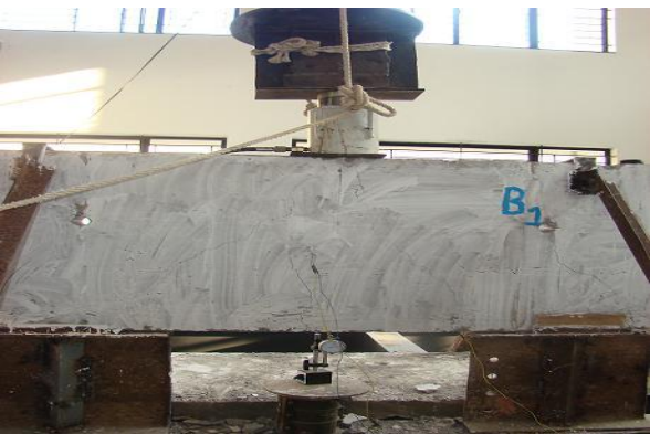
Fig. 7: One Point Loading Test Setup for Deep Beam
