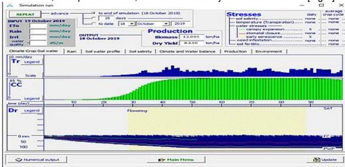
Fig-1 Model generated transpiration, canopy cover and soil moisture in the root zone for treatments T<sub>2</sub>
