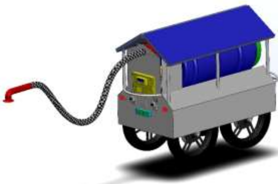
Fig-3 CAD-Solid model of Pneumatic Suction Based Solar Operated Cotton Picker machine
