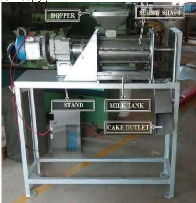
Fig-7 Developed Coconut Milk Extractor
