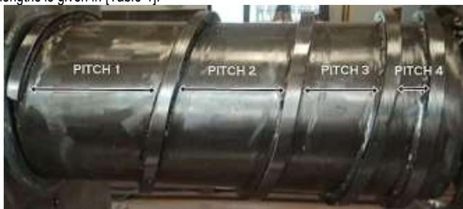
Fig-5 Developed screw press for coconut milk extractor
