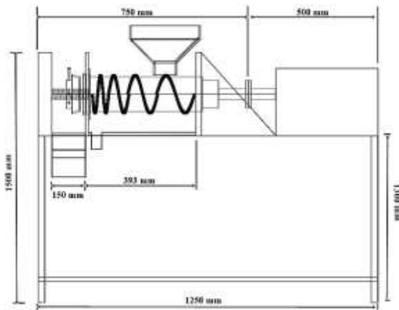
Fig-4 Front view of coconut milk extractor
