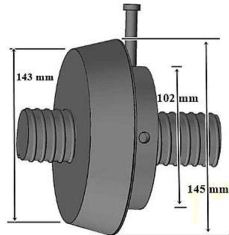
Fig-6 Conical choke
