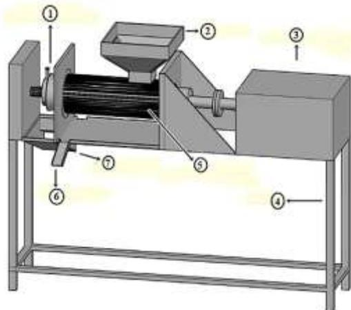
1. Conical nozzle, 2. Hopper, 3. Geared motor, 4. Stand, 5. Screw press, 6. Cake Outlet, 7. Milk Outlet
