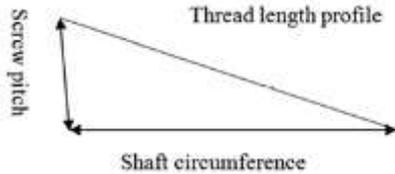
Fig-1 Generation of thread profile
