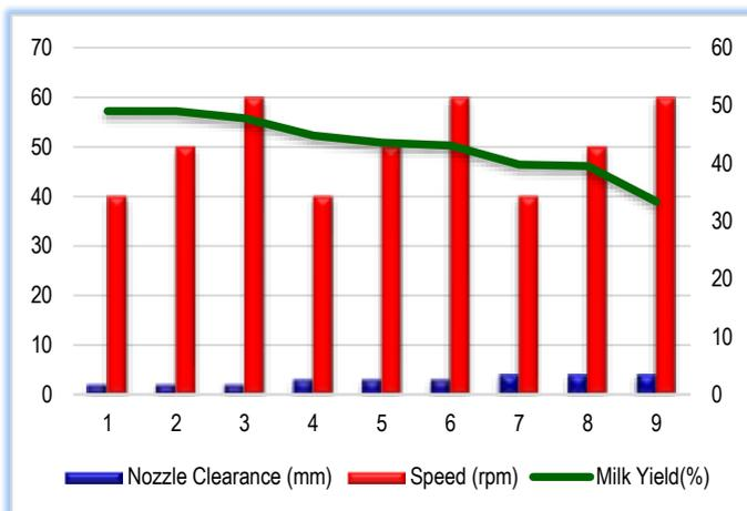
Fig-8 Effect of nozzle clearance and shaft speed on coconut milk yield
