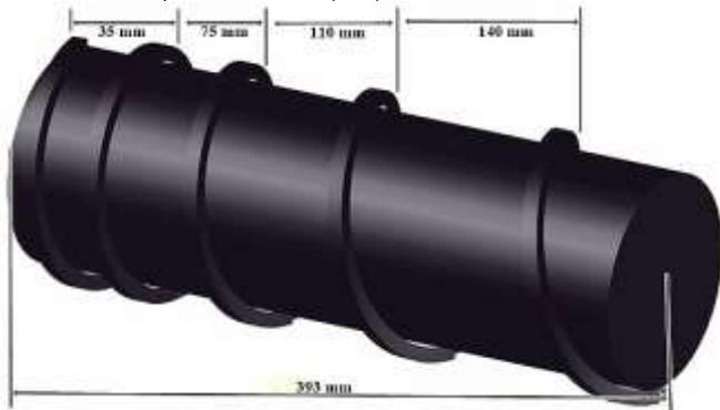
Fig-2 Designed screw press for coconut milk extractor
